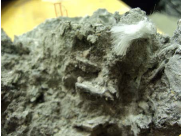
Figure 11. Clump of glass fiber along fracture.
