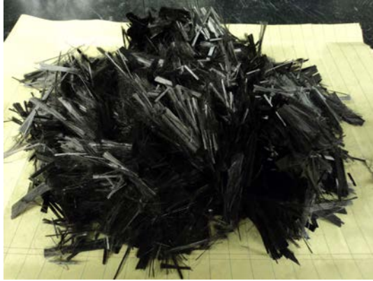
Figure 5. Glass fiber remaining after pyrolysis.
