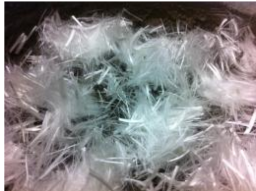
Figure 4. Virgin glass fibers cut from unidirectional strands.
