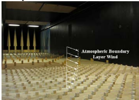
Figure 1. Wind tunnel section with roughness elements
