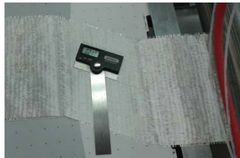
Figure 9: Measurement of deposited shift angle.
