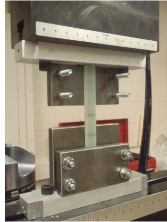
Figure 7. MTS setup for fatigue testing.
