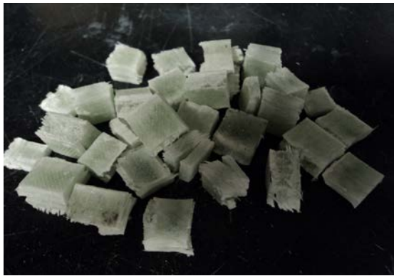
Figure 2. Cubes of Fiberglass Coarse Aggregate.
