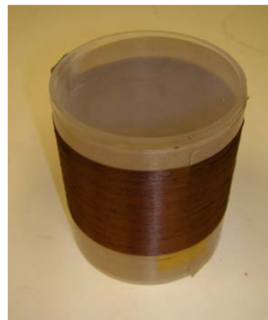
Figure 8 – 1/1 B-lignin/PLA precursor fiber spool
