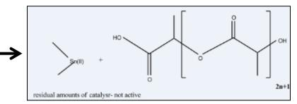
Polylactic acid is graft copolymerized to butyrated lignin hydroxyl group, increasing lignin/PLA miscibility
