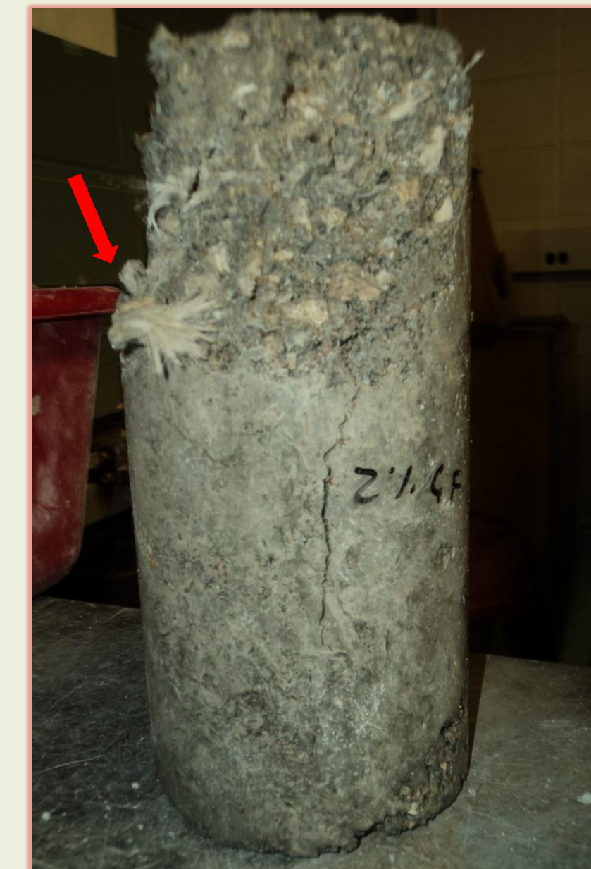
2% fiber test cylinder with fiber clump.
