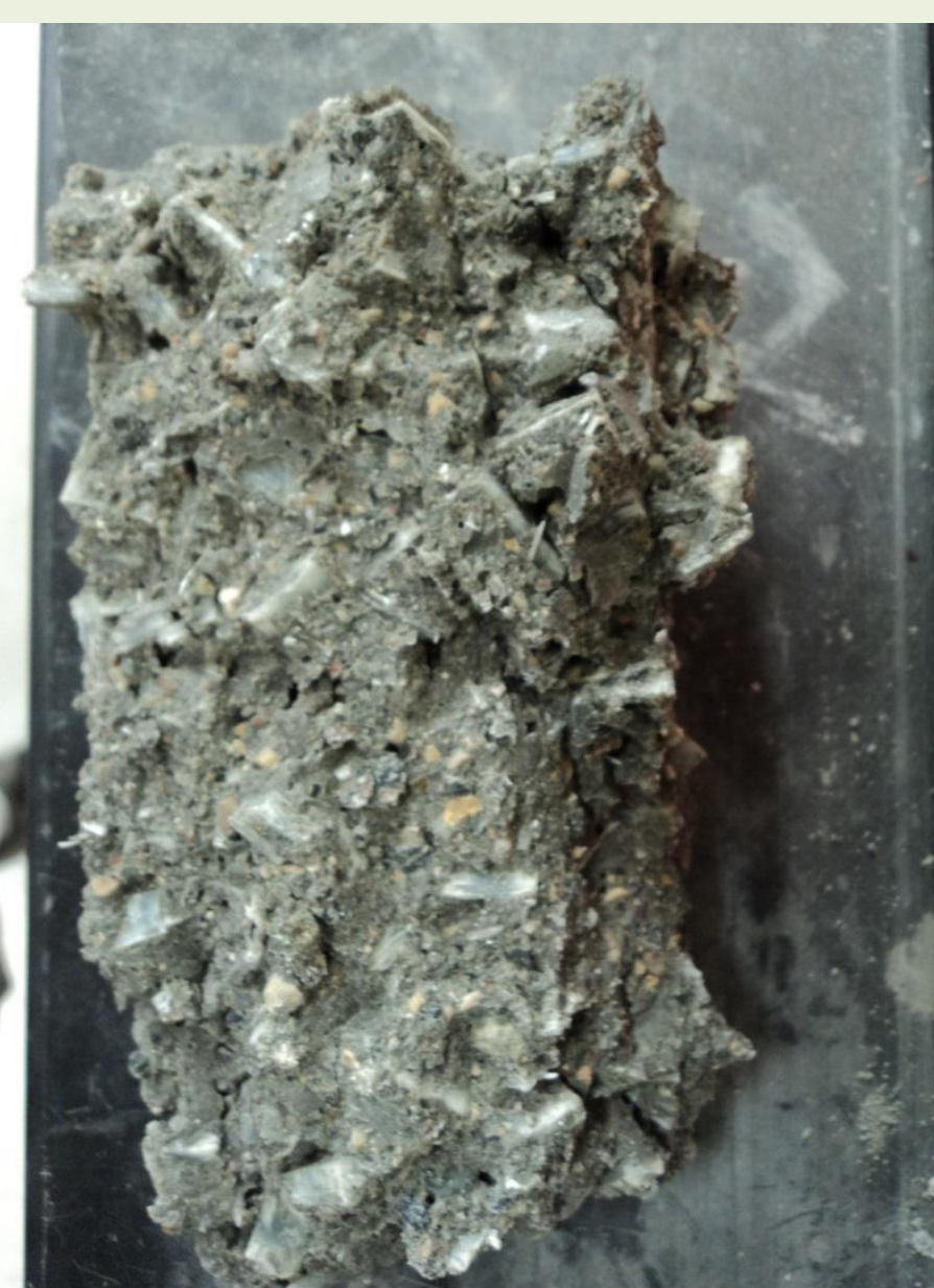
Exposed FRP aggregate cubes
